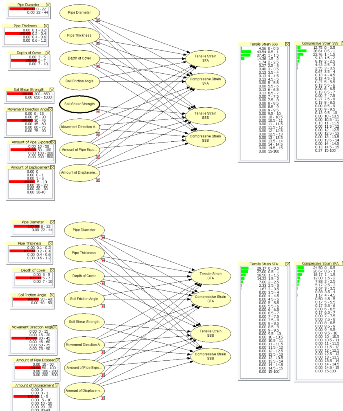
Figure 74: Experienced Strain Model for Lateral Displacement – Tensile and Compressive Strain Calculated Using SSS (top) and SFA (bottom)
